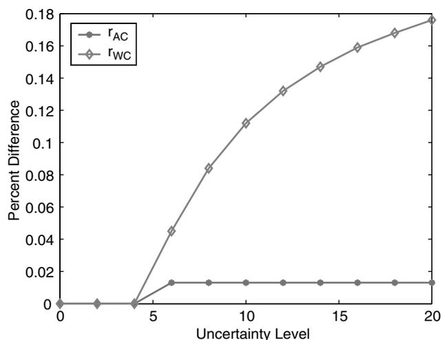
**Figure 2** Relative improvement of solutions as a function of the uncertainty level  $\rho$ , Network 1,  $\mathcal{U}_b$  and  $\mathcal{U}_c$  polyhedral.
