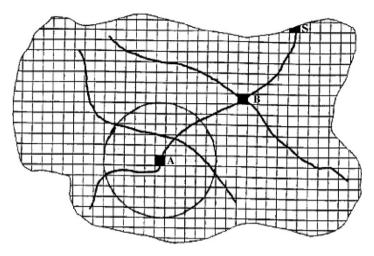
Fig. 2. Network of a harvested area, with A being a machinery location. The circle corresponds to its reach zone. B is an intersection of roads, while S is the exit of the forest.
